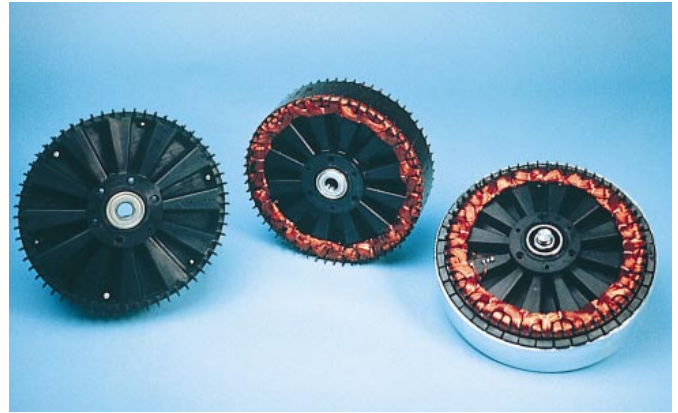
Fig. 35. When used in a washing machine, this very energy-efficient Cadac 1.3-HP (1-kW) DC motor eliminates the need for a gearbox. Stator components in RYNITE® PET are part of an UL 1446 Class F (155°C) Electrical Insulation System.
