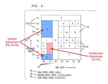
subcarriers), to High-Speed User B [54] that includes frequency bands F0 and F4-F6. In this allocation, the subcarriers in frequency band F0 are non-contiguous with the subcarriers in frequency bands F4-F6. Accordingly, the combination of Ritter, Gesbert, Thoumy, and
