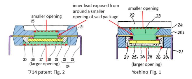
That Yoshino's inner lead is **exposed from around a smaller opening of said package** in the same way as in the '714 patent is shown in the above comparison of Yoshino's Fig. 1 and the '714 patent's Fig. 2, with annotations by Petitioner, and highlighting showing the like elements as described in § III.A. (Ex. 1002, ¶129).
