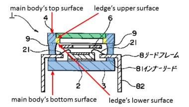
(highlighted blue) **comprises a main body having a top surface and a bottom surface** and **a ledge** (yellow) **formed on said main body so as to extend inwardly toward the center** of the package. (Ex. 1002, ¶273). The ledge holds transparent "cap 5" (highlighted green, although the numeral "5" was omitted from
