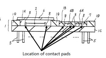
the wire bond connections from the chip, the contacts on each chip are electrically connected to Izumi's package leads:
