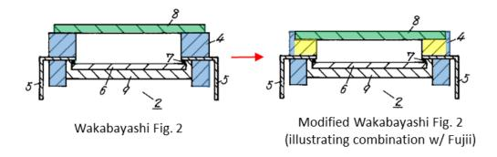
On the right, Petitioner has modified Fig. 2 to show the combination with Fujii, and highlighted the main body portion of the package blue, the ledge yellow, and the transparent lid green. (Ex. 1002, ¶277). Wakabayashi's specification does not indicate what the numeral "8" in Fig. 2 refers to, but, as explained by Mr. Guidash, it is clear that this is a transparent lid, *i.e.*, a "sealing glass", as Wakabayashi recites elsewhere. (Ex. 1004, ¶0002)(Ex. 1002, ¶278).
