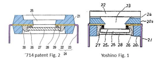
[1d] "a solid-state image sensing device mounted in said package by being inserted from an inlet of said opening which has a wider area, and thereby sealing said through hole, said solid-state image sensing device being secured to said package via an adhesive."
