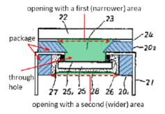
Annotated Figure 1 shows that "the package has openings on both end faces thereof, and different opening areas of said openings." Ex. 1002 ¶ 102; *see* Pet. 16. Dr. Guidash further testifies:
