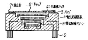
Figure 1 depicts semiconductor chips 4 mounted multi-step-wise in the vertical direction. Ex.  $1022 \, \P \, 9$ . Bumps 3 are formed on the steps where semiconductor chips 4 are disposed. *Id*.
