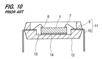
Figure 10 is a cross section of prior art chip 4 mounted in plastic package 12. Ex. 1001, 1:53–56. Lead frame 11 allows for electrical connections to external circuitry and includes inner lead 9 and outer lead 10 molded into
