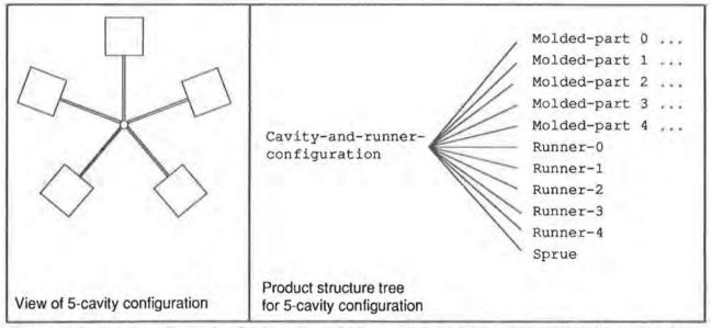
Cavity-and-runner-configuration for 5-cavity mold base. This configuration is optimal for 200 000 parts to mold.
