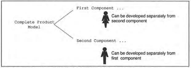
A product model can be modularized using components in a product structure tree.
