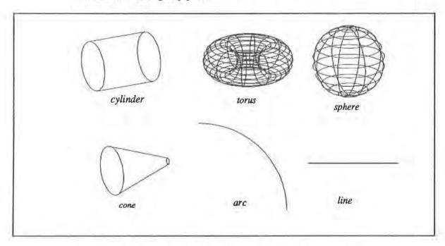
Examples of 2D and volumetric primitives provided by ICAD.
