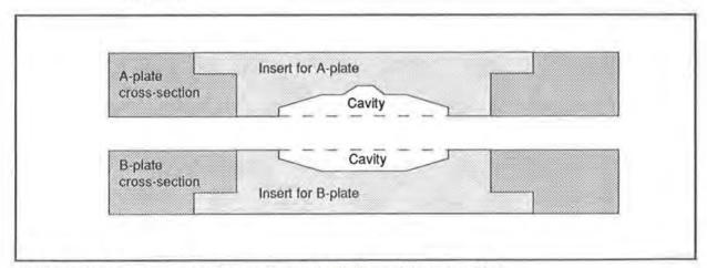
The A- and B-plates contain inserts from which the cavities are milled.
