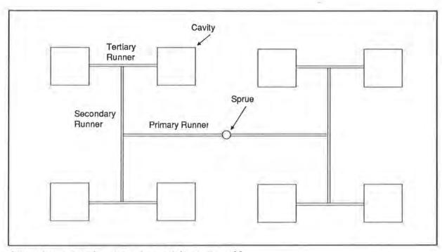
Optimal cavity configuration for an eight-cavity mold.
