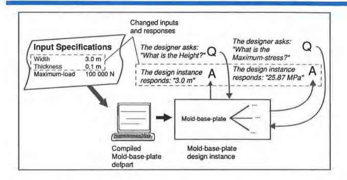
This shows how an ICAD product model can be used to do "what-if" analysis. In this simple Mold-base-plate defpart, you can investigate how the Maximum-stress changes as the input specifications, e.g., the Width, Thickness, and Maximum-load, change.
