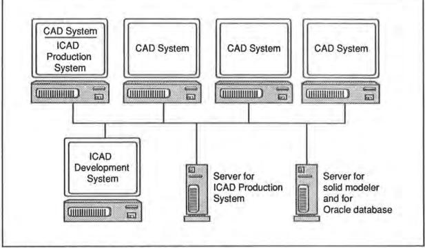
Possible network configuration for the design pipeline.
