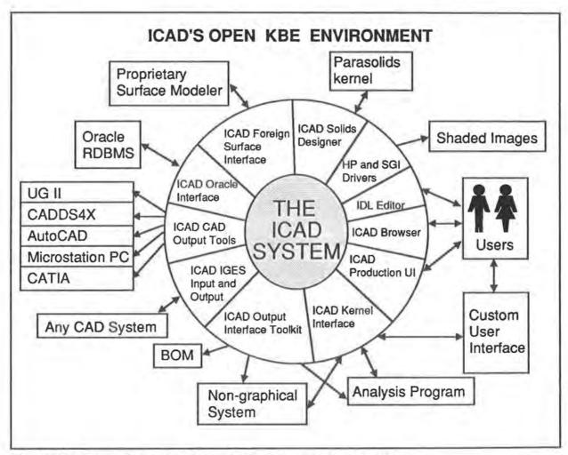
The ICAD System is integrated into an open engineering environment.
