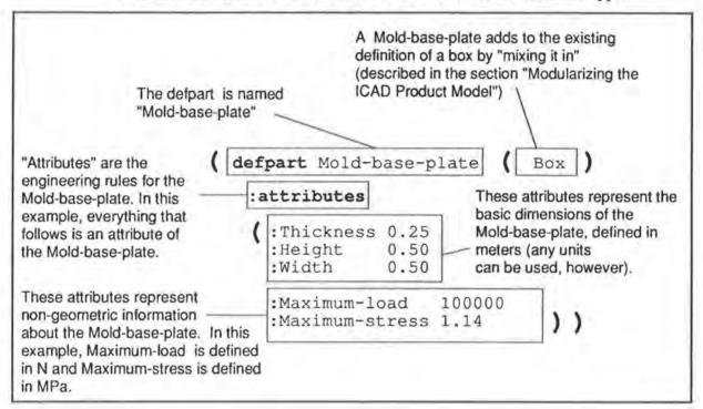
The example starts with a parenthesis which indicates that a new defpart is being defined. The word **defpart** indicates that the name and definition of the defpart follow.
