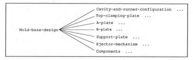
If we want to look at one of the children of the mold base in detail, we can ask The ICAD System to expand that portion of the tree. In this case, we ask to expand the Top-clamping-plate, and we find that the Top-clamping-plate has six children. One child, the Plate, represents a box with the same dimension as the Top-clamping-plate. The five other children represent holes in the Top-clamping-plate.
