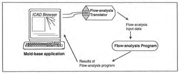
Mold-base product model output to flow-analysis package. The analysis result is read back into the ICAD product model as system inputs, forming a closed loop.
