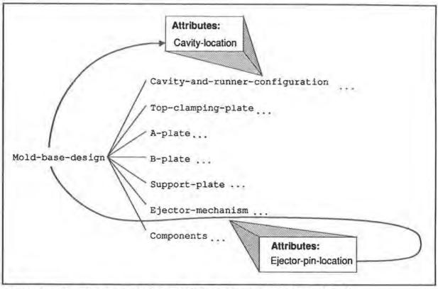
The Ejector-pin-location attribute in the Ejector-mechanism part depends on the Cavity-location attribute in the Cavity-and-runner-configuration part.
