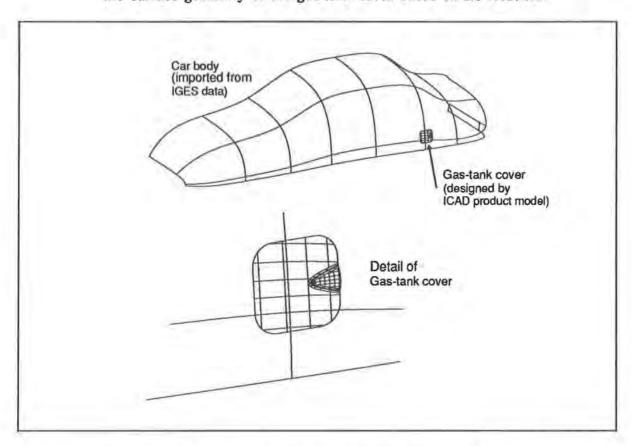
View of a gas-tank cover that is automatically generated by an ICAD product model. The geometry for the automobile body is imported via IGES.
