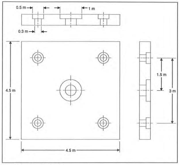
CAD drawing of top clamping plate.
