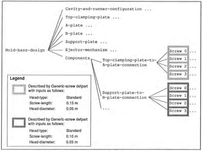
The mold base uses different kinds of screws, each described by the same generic-screw defpart with different inputs. In this product structure tree, the screws used to hold the Top-clamping-plate to the A-plate are different than the screws used to hold the Support-plate to the B-plate.
