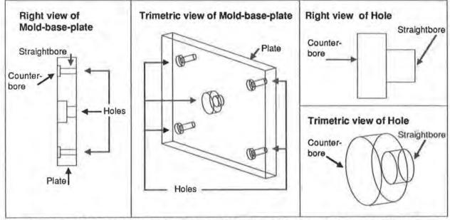
Drawing of the Mold-base-plate with components labelled. Also shown is a drawing of a Hole, which includes a Counterbore and Straightbore. The different parts are modeled using ICAD-provided geometric primitives.
