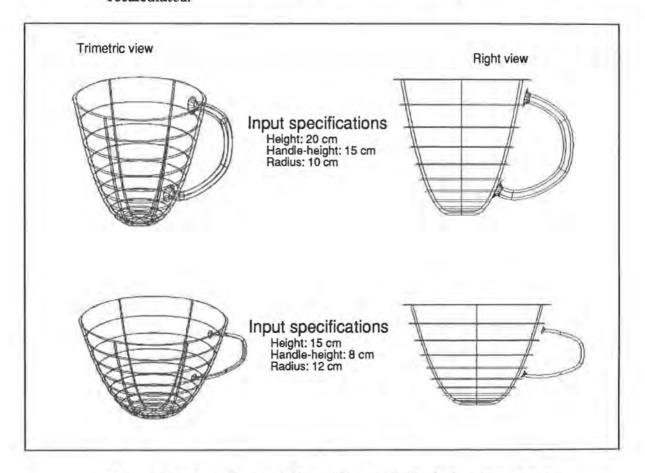
Trimetric and right view of two different design instances of a cup. As the input specifications change, the surface definitions (fillets, sweeps, revolutions) are automatically updated.
