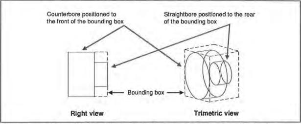
Counterbore and Straightbore positioned inside a Hole assembly, whose bounding box is indicated using dashed lines.
