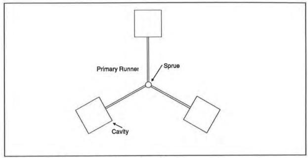
Optimal cavity configuration for a three-cavity mold.
