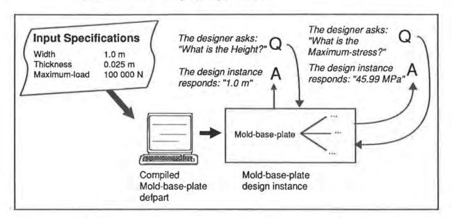
Another set of inputs creates a new design instance which has a different value for Maximum-stress. The following inputs to the Mold-base-plate defpart, for instance, produce a new value for Maximum-stress:
