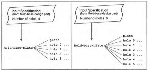
A Mold-base-plate has five components when the input Number-of-holes is four, and seven components when Number-of-holes is six.
