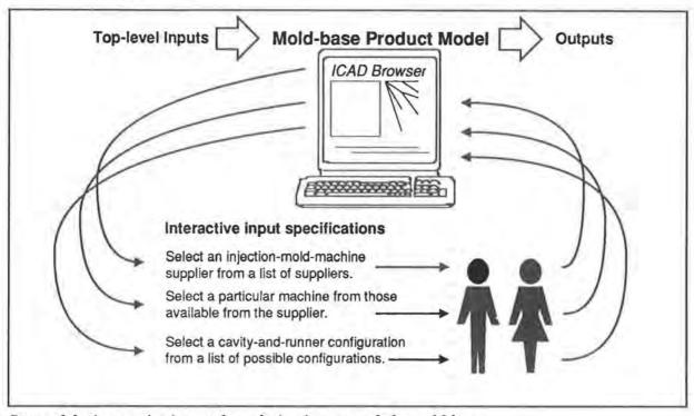
Some of the interactive inputs for a design instance of the mold base.
