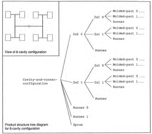
Cavity-and-runner-configuration for 8-cavity mold base. This configuration represents the optimal configuration for 3 000 000 parts to mold.
