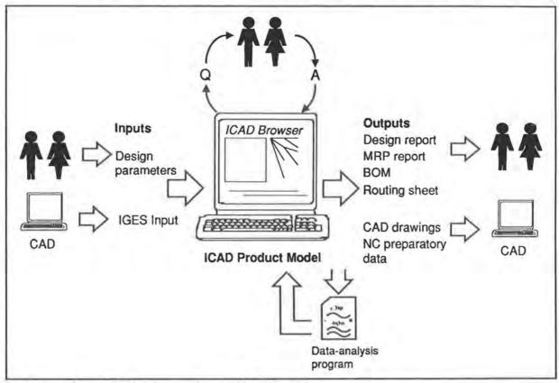
Design pipeline including interaction with design engineer.
