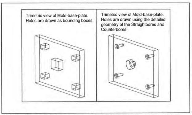
Mold-base-plate. On the left, just the bounding boxes of the holes are drawn. On the right, the detailed geometry of the holes, that is, the Straightbores and Counterbores, is drawn.
