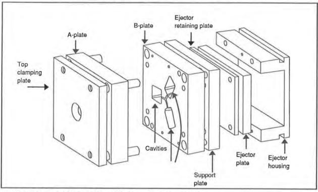
Exploded diagram of a mold base with the components labelled.
