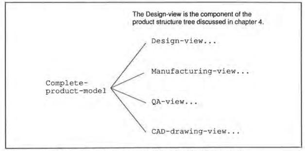
Different views of the same product are represented in the product structure tree using a different component of the root to model each view.
