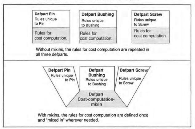
Often mixins are used to divide the information that would normally be in a single defpart into separate defpart modules. A single defpart that includes hundreds of attributes would be tiresome to write, hard to read, and difficult to maintain. Instead, the different attributes are divided into logical categories, and the attributes in each category are defined in separate defparts.
