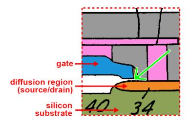
'924 patent (admitted prior art) at Fig. 2B, 2:15-20 ("a polysilicon gate 32 is first formed without direct contact with the diffusion regions 34 and 36 in a silicon substrate 40.") (Ex. 1101); Decl. ¶ 87 fn.6 (Ex. 1102).
