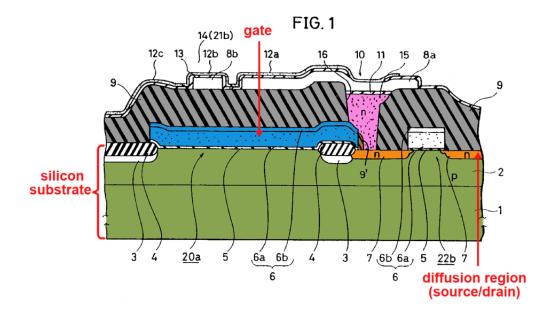
Sakamoto at Fig. 1, 6:52-58 ("A plug layer 15 of polycrystalline silicon directly connected to the n+ source/drain region 7 and gate electrode 6 is embedded within opening 16."), 7:17-32 ("a silicon substrate 1 … form gate electrodes 6, 6 of MOS transistors 20a, 22b…") (Ex. 1103); *see also id.* at claim 1, 2:23-32, 4:20-67, 6:39-7:7, 7:17-52, 12:57-58. Decl. ¶ 85 (Ex. 1102).
