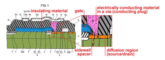
Sakamoto at Fig. 1, 7:44-52 ("a sidewall spacer 9" is located in the "opening 16"), claims 6 and 9 (Ex. 1103).<sup>9</sup> Decl. ¶ 88 (Ex. 1102).
