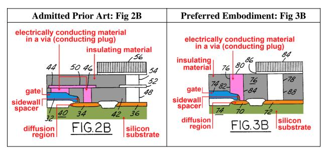
As shown in Figures 2B and 3B, in both the admitted prior art of the '924 patent and the allegedly novel structure, the gate is connected to the diffusion region (source or drain), by either two connected plugs, or a single plug. The diffusion region is located in a substrate and is not directly connected to the gate. The gate is substantially covered by an insulating material. Decl. ¶ 49 (Ex. 1102).
