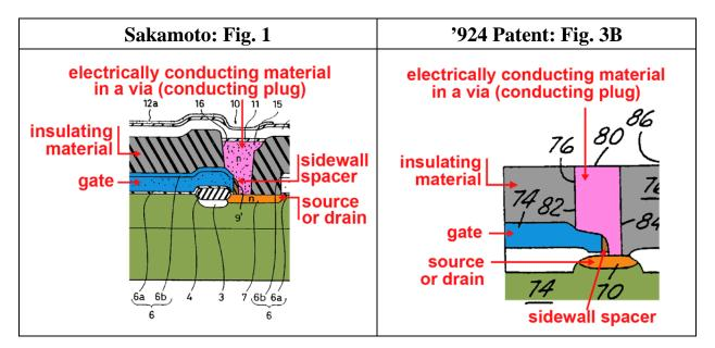
As shown, both structures include a gate connected to a source or drain
