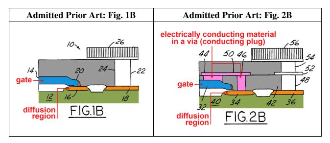
The '924 patent acknowledges that both examples were known prior art. *See* '924 patent at Figs. 1A, 1B, 2A, 2B, 1:25-2:45, 3:30-35 (Ex. 1101); Decl. ¶ 43 (Ex. 1102).
