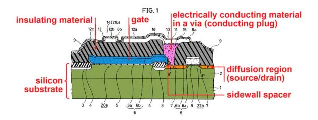
Sakamoto at Fig. 1, 6:39-8:52 (describing Figure 1), claims 1-9, 3:55-57 (an "object of the present invention is to provide a method of manufacturing an
