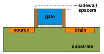
As was known as of the time of the alleged '924 invention, such sidewall spacers help to prevent direct electrical contact between the gate electrode and nearby components and thus help to prevent short-circuits. Decl.  $\P$  40 (Ex. 1102).
