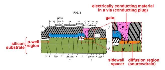
Sakamoto at Fig. 1 (Ex. 1103); *see also id.* at Figs. 2-5, claims 1, 4, and 7, 6:49-7:14 ("An opening 16 is formed in an interlevel insulating layer 9 .... A plug layer 15... directly connected to the n+ source/drain region 7 and gate electrode 6 is embedded within opening 16."), 7:15-8:12 (plug layer 15 is formed when
