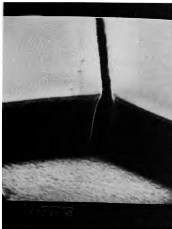
FIG. 8. Submicron trench for a Ga As gate obtained using a Kasper 10:1 step and repeat camera for the top layer. (SEM photo).
