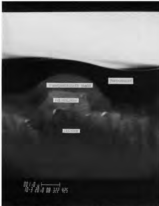
FIG. 1. X-ray resist thickness variation as it steps over 1.0\text{ }\mu\text{m} of p -glass flowed over a 1.0\text{ }\mu\text{m} high poly-silicon feature. Resist varies from 0.8\text{ }\mu\text{m} on top of the feature to 1.7\text{ }\mu\text{m} in the valley between features (SEM profile photo).
