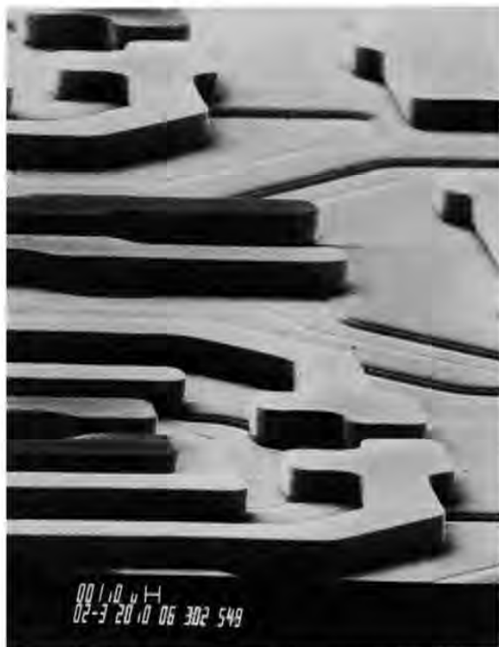
FIG. 11. Application of the trilayer resist to reactive ion etching of 0.65\ \mu\text{m} of polysilicon on a device wafer. The thick resist is still on and is used as the etch mask.
