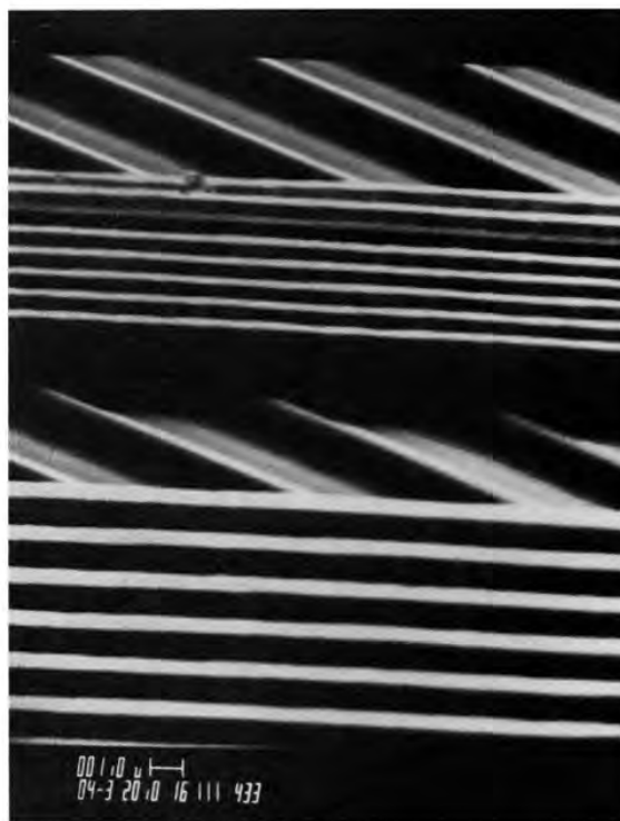
FIG. 10. (a) 1.0\text{ }\mu\text{m} lines and spaces in thick resist, using x ray for the top layer. The lines are traversing a 1.0\text{ }\mu\text{m} high, periodic grating to demonstrate good step coverage with no linewidth variation over steps (SEM photo). (b) Profile of the wall of resist for one of the 1.0\text{ }\mu\text{m} lines showing conformal coating of the wafer topology at the resist bottom and a flat surface at its top (SEM photo).
