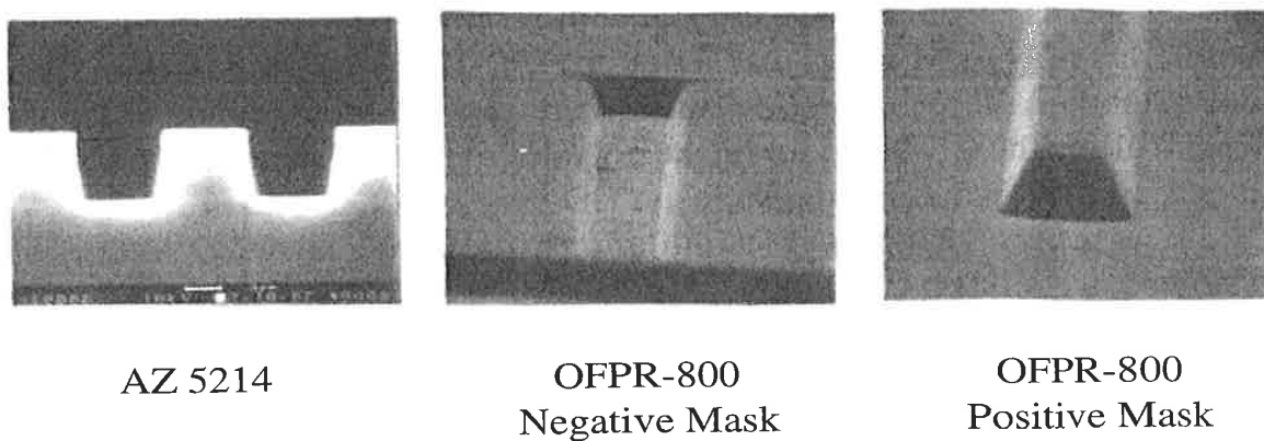
Figure 116. Edge wall profiles for conventionally developed positive photoresist images. Note, the edge walls are poorer than those for both IREV processes.
