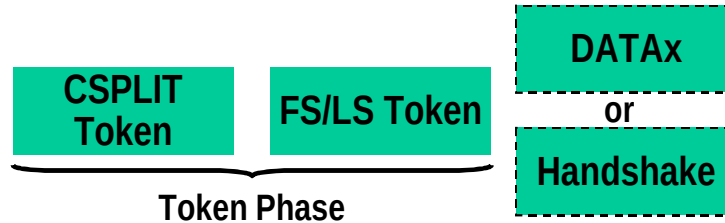
Figure 8-7. Packets in a Complete-split Transaction
