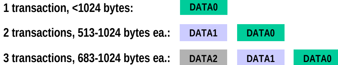
Figure 5-11. Data Phase PID Sequence for Isochronous IN High Bandwidth Endpoints
