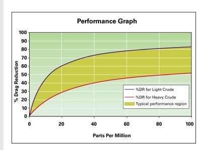
The performance curve shows the performance range in which LP 300 Flow Improver operates, depending on pipeline and crude conditions.
