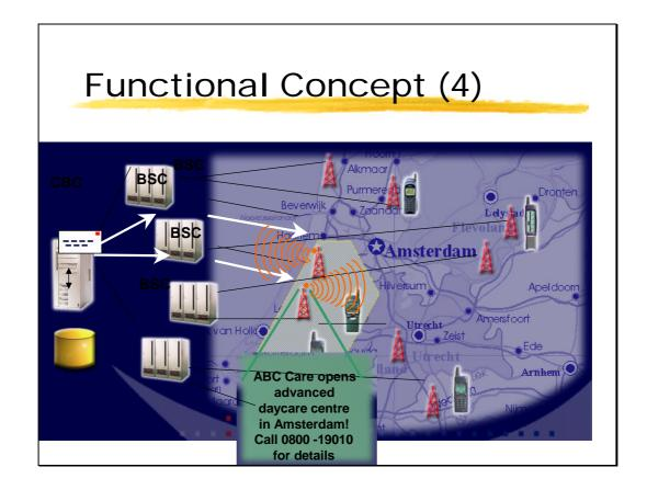
The CBC receives the geographical definition of the broadcast area from the content provider, selects the relevant base stations for the area and stores the CB message until the specified start time arrives. Or, if the content provider has specified that broadcast must start as soon as possible, the CBC starts the broadcast immediately.
