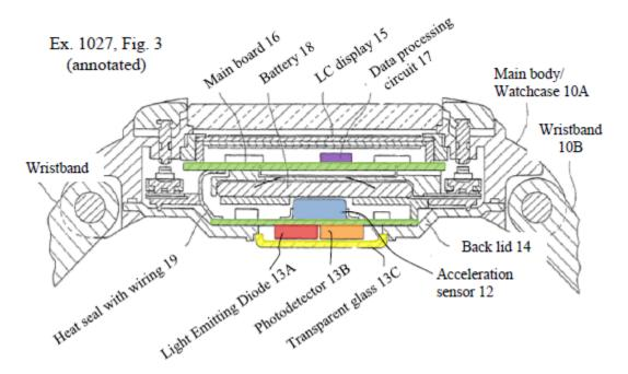
Pet. 16. Figure 3 depicts device main body 10A, including back lid 14 and transparent glass 13C, which is held against a subject's wrist (not shown) by wristband 10B. Ex. 1027 ¶ 140. "The transparent glass 13C is fixed by means of a back lid 14 as a component of the device main body 10A." *Id.* ¶ 141. The reverse side of main body 10A includes pulse wave sensor 13 and acceleration (body motion) sensor 12. *Id.* ¶ 140.
