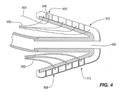
Figure 4 depicts a section of first end 112 of conductor portion 104 for insertion into the wearer's auditory canal. Ex. 1031 ¶¶ 22, 33. Fiber optic cables 402 terminate in optically transparent elastomer 408 of first end 112 to allow the communication of light between fiber optic cable 402 and the auditory canal wall. *Id.* ¶ 33.
