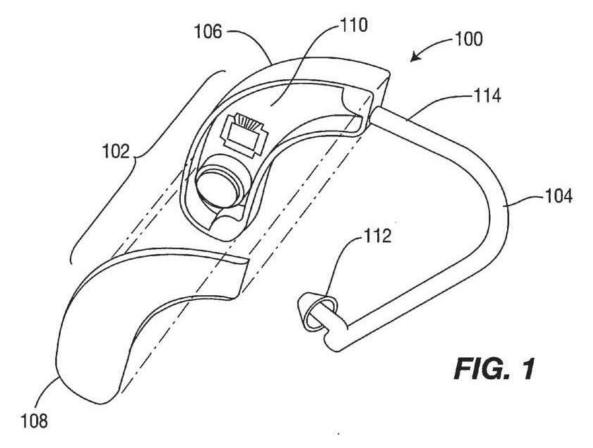
Figure 1 depicts a partially exploded view of an exemplary monitoring device in accordance with Aceti's disclosure. *Id.* ¶ 7. Monitoring device 100 includes processor portion 102 and conductor portion 104. *Id.* ¶ 16. In
