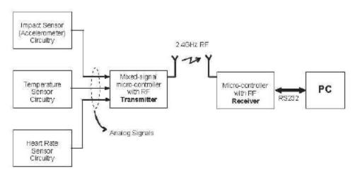
Fig. 1. Functional block diagram of the system hardware
