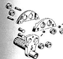
Fig. 9: Centrifugal pendulum absorber with bifilar suspension on the crankshaft of an aircraft engine (R1820 Cyclone) from Pratt & Whitney [6]
