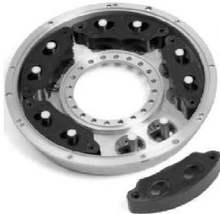
Fig 12: Centrifugal pendulum absorber with bifilar suspension in the flywheel [7]
