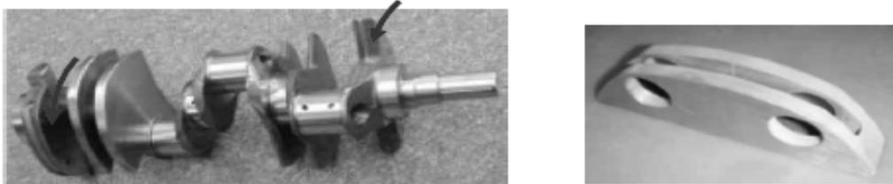
Fig. 10: Crankshaft used in the engine with two pendulum attached (left) and one of the pendulum absorbers used on the crankshaft (right), Ford Motor Co [6]
