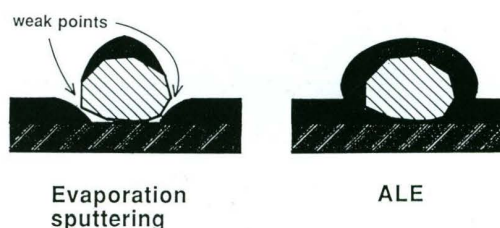
Fig. 5. Effect of saturated surface coverage on pinhole formation under microcontamination particles.
