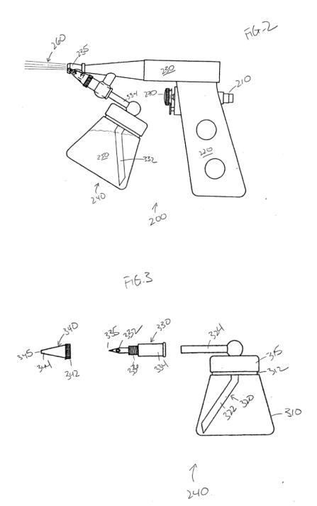
The cell spray apparatus of Dixon "comprises gas inlet 210, handle 220, barrel 230, reservoir assembly 240, and trigger mechanism 270."). Dixon further discloses that "when trigger mechanism 270 is depressed, pressurized gas is
