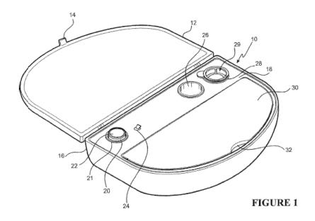
Located within the base portion **16** is a first member **18** within which there is provided an aperture **20** in which there is located a vial **22** for the enzyme.
