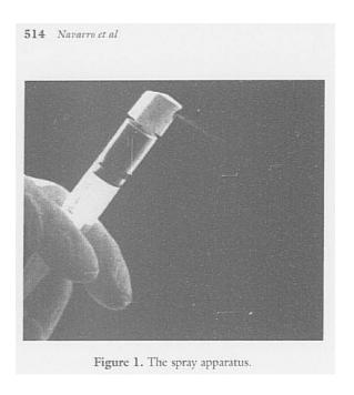
(Ex. 1003, p. 514.) Navarro tested syringe and nozzle combinations that failed to provide a spray: "[n]ozzles were eliminated if the droplets were too large and just
