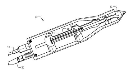
14. The apparatus may comprise a first member, not shown, and second member 10 wherein: the first member includes power supply, gas/air supply and electronic controls, and the second member 10 includes a sterilizeable spray head 12 and a container 14 with the cell suspension 16. In that case both members may be connected through connectors 18, 20. One connector may supply power and the other connector may supply gas/air from the power supply and gas/air supply
