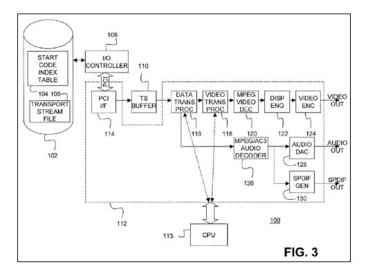
*Id.* at Figure 3. MacInnis also states that the CPU's DTD can use the command packets to send "various commands" to the video decoder 120, but does not expressly state what those commands are or how they affect the system. *Id.* at
