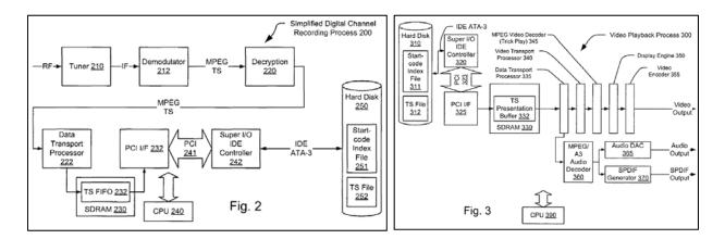
Ex. 1001, Figures 2, 3. Whereas Chen '677's system does not include a central processor responsible for the overall control of the system, as shown in Figure 3 below.
