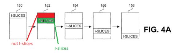
Figure 4A of MacInnis (annotated) illustrates changes to the location of I-slices in a block of pictures without I-pictures. Ex. 1003 ¶ [0018]. The I-slices move down until all rows in the consecutive sequence of pictures have been represented in I-slices. Pet. 19 (citing Ex. 1003 ¶¶ [0056]–[0057]). MacInnis also describes a system for implementing reverse play. *Id.* ¶¶ [0108]–[0119]; Pet. 19–23.
