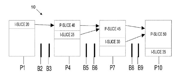
Figure 1 of Chen '677 shows a video stream where the I-frame is divided into slices and spread across P-frames. Chen '677 explains that those skilled in the art will appreciate that the P-frames need only be partially decoded in order to recover the I-slices. *Id.* ¶ [0025]. Reconstructing a P-frame requires decoding at least the previous frame. *Id.* ¶ [0022]. For example, I-slice 25 and P-slice 40 in P-frame P4 provide
