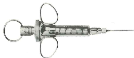
STATHAM INSTRUMENTS INC. - MODEL SP25 OVERALL LENGTH \approx 9" OUTPUT WITH 7.5VRMS EXCITATION = 37\mu VRMS/mmHg
