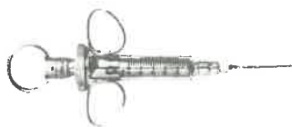
STATHAM INSTRUMENTS INC. - MODEL SP25 OVERALL LENGTH = 9" OUTPUT WITH 7.5VRMS EXCITATION = 37 \mu VRMS/mmHg
