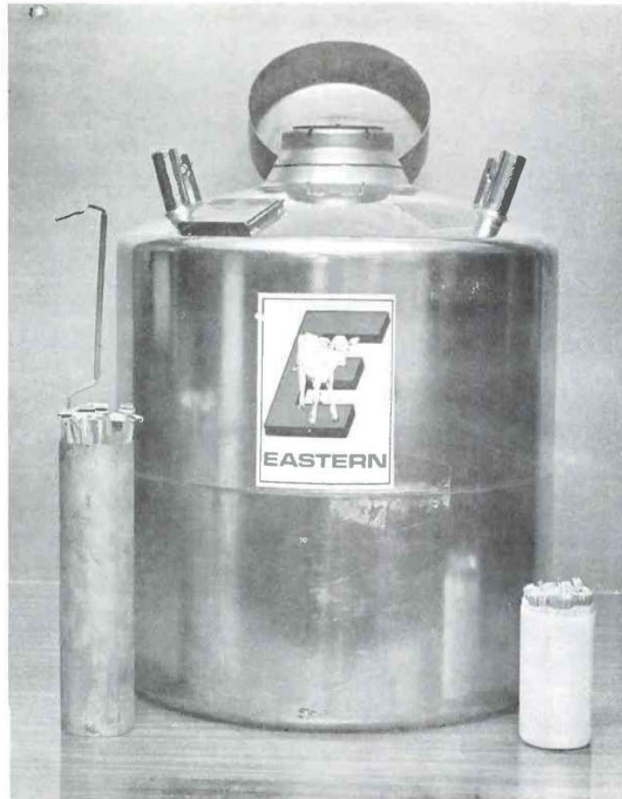
Figure 17.5 — A liquid nitrogen (LN) straw and ampule storage container. The ampules fixed to metal “canes” are suspended in cannisters (see at left). Straws are placed in goblets and in a container (shown at right) for suspension in the LN refrigerator. (Photo courtesy Eastern Artificial Insemination Cooperative, Ithaca, New York)
