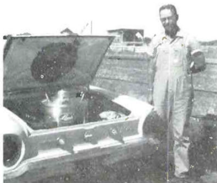
Figure 17.8 — Showing raised section of car trunk — necessary for some cars to accommodate liquid nitrogen container.
