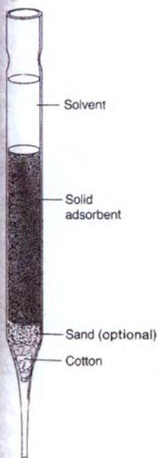
FIGURE 12-7. Microscale chromatography column
