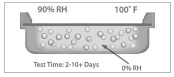
During the gravimetric test, a cup or dish is filled with desiccant or water, placed in a temperature and humidity controlled chamber, and weighed periodically. Depending on the barrier properties and sample thickness, the gravimetric method could require a test time of one day to two to three weeks (or longer). Enough data points should be collected until weight gain (or
