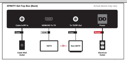
In the figure above, the XFINITY set-top box includes a "Cable In/RF In" Connection connected to the Comcast network via coaxial cable to receive television input signals and send return signals. Set-top boxes receive first output (compressed voice data) from remotes via RF and transmit second output (uncompressed voice data) to a central processing station via the coaxial cable connection.
