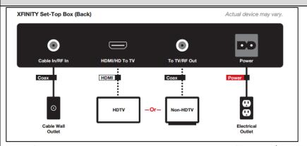
In the figure above, the XFINITY set-top box includes a "Cable In/RF In" Connection connected to the Comcast network via coaxial cable to receive television input signals and send return signals. The XFINITY set-top box also includes connections to television sets to provide output signals. Set-top boxes receive first output (compressed voice data) from remotes via RF and transmit second output (uncompressed voice data) to a central processing station via the coaxial cable connection.
