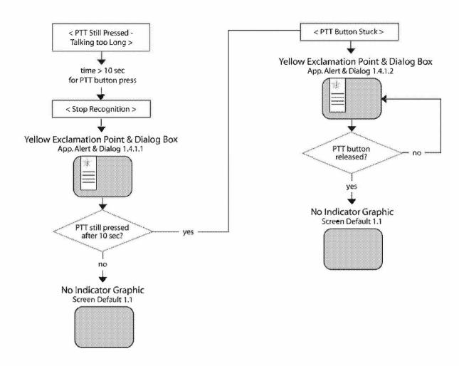
There are two different messages when the talk button is held down for a long interval. The first message covers the relatively normal case where the cable subscriber takes more than ten seconds to speak the command. The second covers the abnormal case where the PTT button is stuck. There is no transition between the two messages. The second message stays on screen until the button is released.
