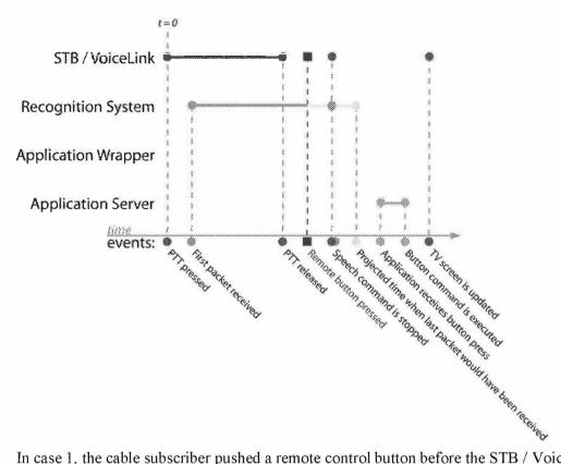
In case 1, the cable subscriber pushed a remote control button before the STB / Voice Link sent all of the packets for the speech command to the Recognition System. The diagram shows that the speech command is cancelled and the remote control button command is executed. The STB / Voice Link and the Recognition System should cooperate to cancel the speech command.
