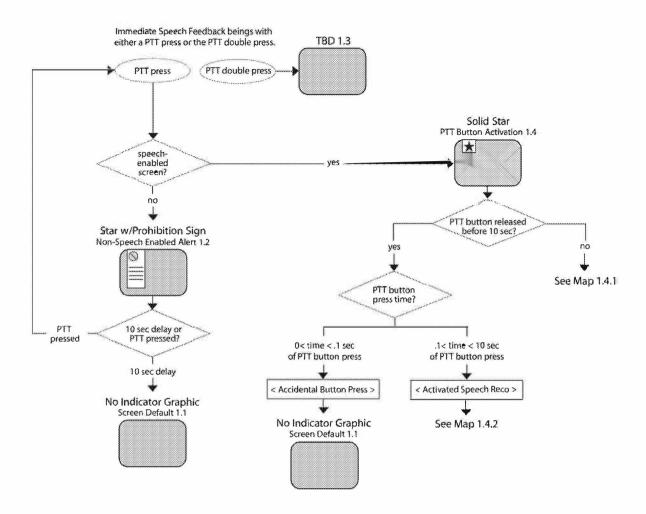
Note that the preceding flowchart includes a double press of the talk button. The action to be taken when this is detected is still TBD. A double press has occurred when there is 400 ms or less between the "key-up" of a primary press and the "key down" of a secondary press.
