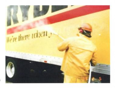
(Above) The 4075D's power is controllable, making the removal of decals or single layers of paint possible.
