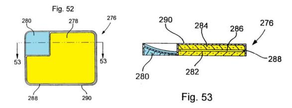
Petitioner's annotated Platzer Figures 52 and 53 depict a rearview mirror assembly. As seen from the above, Platzer Figures 52 and 53 show a magnification region 278 and a second magnification mirror 280 for viewing primarily the blindzone. Ex. 1013, 37:20–22. The second mirror is "placed in the upper and outer quadrant of the rearview mirror." *Id.* at 15:16–17.
