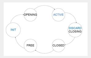
The most important state in the life cycle is the Active state. From Active state, the session will transition to either the Discard or Closing state based on the following conditions:
