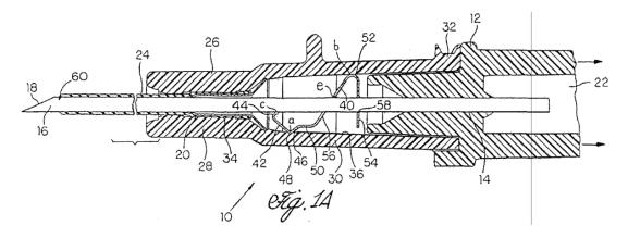
Woehr describes Figure 1A as depicting catheter 10 including needle hub 12, needle 16 with needle tip 18, catheter hub 26, and needle guard 40 in the form of a unitary spring clip. *Id.* at 4:8–28, 50–51. Functionally speaking, as needle 16 is withdrawn from a patient, needle guard 40 "automatically snaps into a retracted position" to block needle tip 18 to prevent accidental contact to the health care practitioner. *Id.* at 4:43–49.
