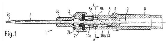
According to the '762 patent, Figure 1 depicts catheter insertion device 1 with catheter 4, needle hub 8, to which hollow needle 9 is fixed and which needle 9 passes through valve disc 7 and extends through catheter 4.
