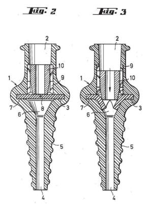
Tauschinski's Figures 2 and 3 depict a connector with a slit sealing disc. *See id.* at 2:62–68. In particular, these figures depict member 10 slidable within hollow-conical portion 2 and disc 3 provided with central slit 8. *See id.* at 3:17–25. Figure 2 depicts disc 3 as closed, with Figure 3 depicting member 10 advanced downward and within slit 8 of disc 3 to open the slit. *See id.* at 3:29–36.
