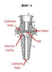
Petitioner asserts that Tauschinski discloses valve 3 with slit 8 configured to obstruct fluid flow through catheter hub 1. *Id.* at 15-16 (citing in-part Ex. 1005, 3:14-19). Petitioner reasons that it would have been obvious to modify Woehr "by adding protective elements, such as a valve to prevent the emergence of blood," as disclosed by Tauschinski. *Id.* at 17 (citing Ex. 1002 ¶¶ 63-68).
