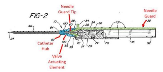
Figure 2 of the catheter hub assembly from Van Heugten, above, and as annotated by Patent owner, illustrates in green a portion of the needle guard and, in blue, the catheter hub.
