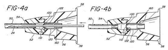
As disclosed in Van Heugten, Figures 4a and 4b further show membrane assembly 100 comprising a one-directional valve membrane 110. *Id.* at 3:59–64. Figure 4a (above-left) depicts membrane 110 as being "punctured" by needle 24 (*id.* at 3:59–4:3), while Figure 4b (above-right) depicts needle 24 removed, where upon "removal from the catheter hub 52, the valve membrane closes" (*id.* at 4:6–9). The sealed valve member 110 is "generally configured as a 'duck bill' valve or a valve of similar
