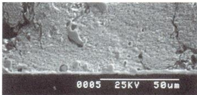
Figure 13-5. Bonding layer between solder and the substrate.
