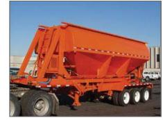
feed gate control valves, hydraulic reservoir and quick disconnects are included in our scope. Flood lights are provided near the discharge end, and at the operators' station for night time service. Load the trailer with frac sand by gravity chutes, or with mechanical conveyors, or pneumatic conveyors. The trailer is equipped with a top side walkway, access ladders and a fold down handrail system.
