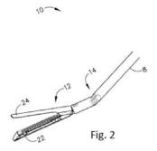
The articulation joint allows the shaft to articulate along two axes. Articulation cables couple the articulation joint to the tool mounting portion, such that the articulation joint may be operated by rotary motion from the robotic system. The '969 patent also contains tactile feedback sensors in the end effector.
