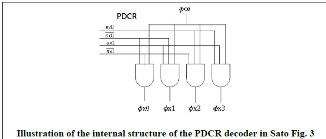
Ex. 1003 ¶ 62. The figure reproduced above is captioned "Illustration of the internal structure of the PDCR decoder in Sato Fig. 3." Ex. 1003 ¶ 62. In support of his testimony, Dr. Horst cites a textbook titled *Fundamentals of Digital Logic with Verilog Design* (Ex. 1009) that shows how a truth table for a decoder is implemented using AND gates and inverters. Ex. 1003 ¶ 63 (citing Ex. 1009, 312 (Fig. 6.16), 315).
