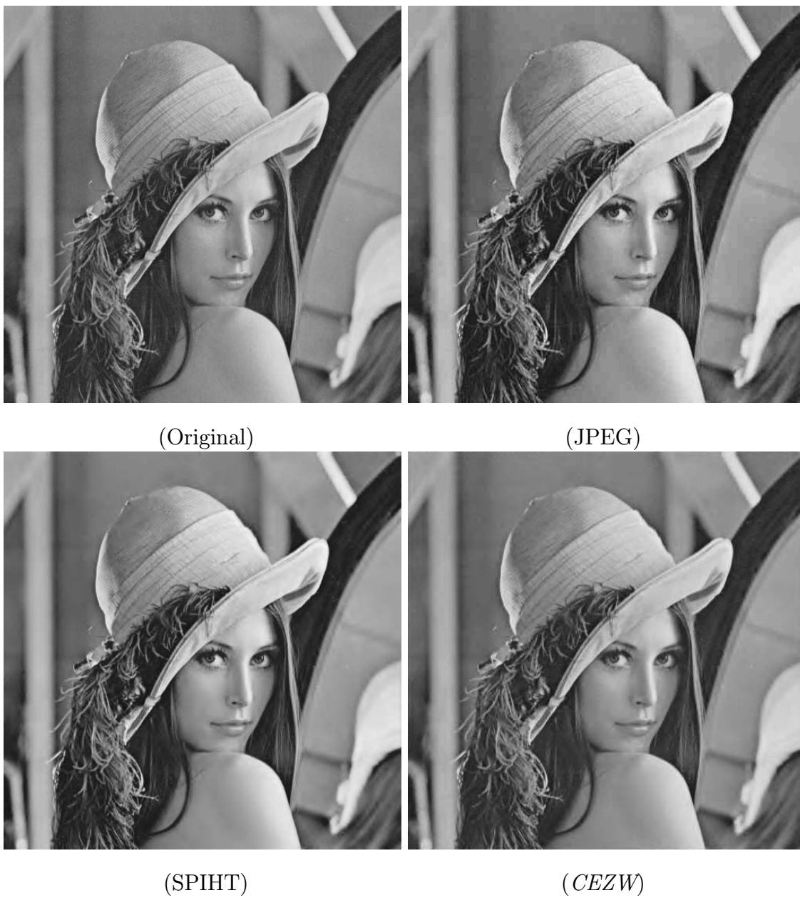
Fig. 5.8. The original and the decoded images of Lenna at 0.5 bpp using CEZW , JPEG and SPIHT.
