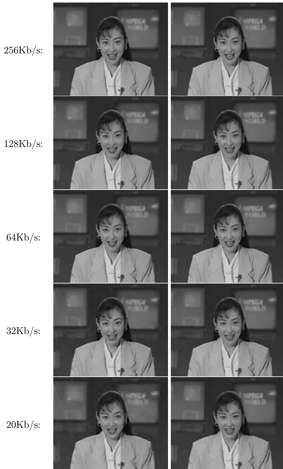
Fig. 6.11. Frame 78 of the Akiyo sequence (QCIF, 10 frames per second), decoded at different data rates. Left column: SAMCoW , right column: H.263.
