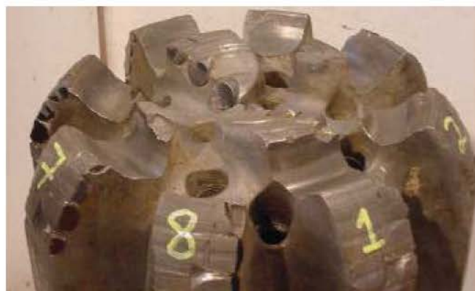
Figure 13a. BD548 in Worn state showing signs of classical stick slip 5
