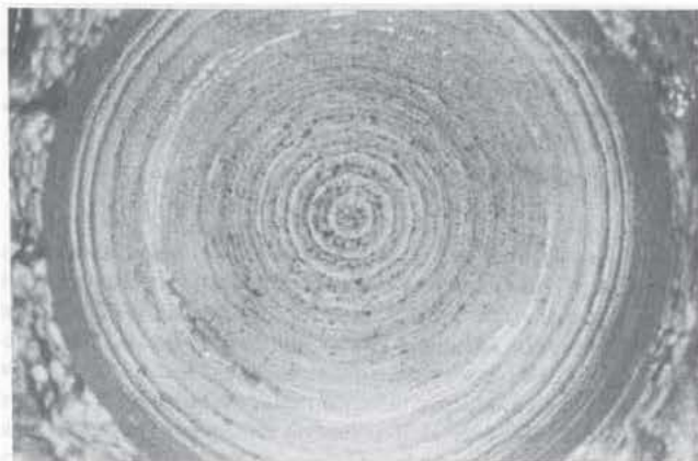
Figure 7 - Bottomhole patterns generated while drilling Carthage limestone. The left one was drilled with the 16 in. Anti-Whirl PDC bit. The right one was drilled with a 12-1/4 in. conventional PDC bit.
