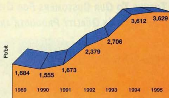
Fig. 5. Since 1989, PDC bit life has increased 115% to an average of 3,629 ft by mid-1995.
