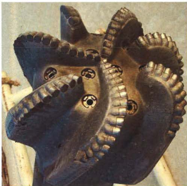
Figure 23: Dull condition of PDC-B, after run in West Kuwait (Minagish Field). The bit established a new field record, and performed as predicted, giving credibility to the engineering processes used in its development.
