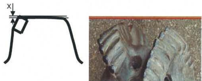
Figure 3: Impact damage to PDC cutters, as a result of severe bit vibrations.
