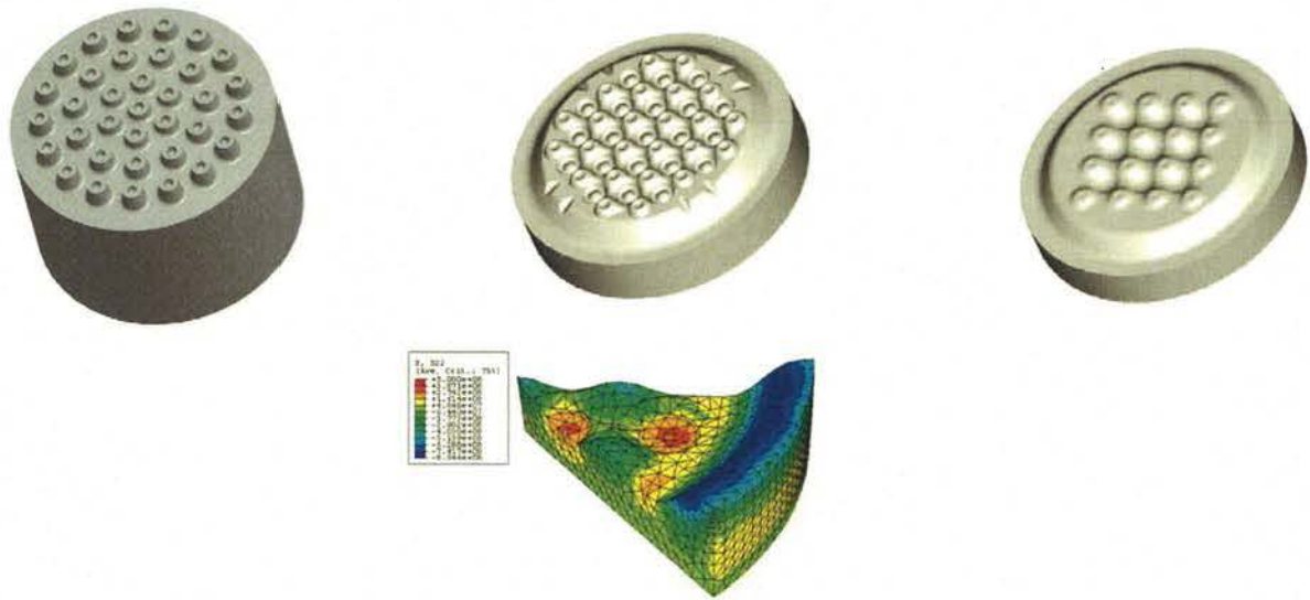
Figure 20: Carbide interface geometry (CIG) development through FEA analysis. The process is used to enhance impact resistance by reducing damaging residual stresses and their gradients.
