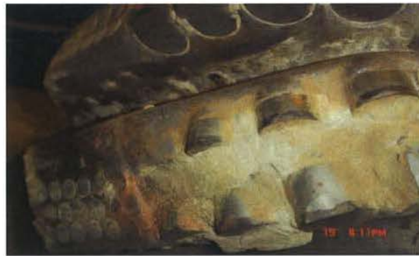
Figure 9: Packed cuttings (formation) between cutters on double row (back-up blade) bit. Inability to clean cutters on second row, due to inefficient nozzle layout, compromises bit performance, especially in soft (fast drilling) formations.
