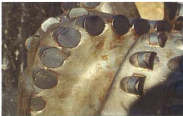
Figure 8: Dull condition of double row PDC bit. The increased blade deployment and resulting higher total cutter count drastically increases total wear flat area, even at low wear conditions. This condition has a huge negative effect on ROP, especially in hard and/or abrasive formations.
