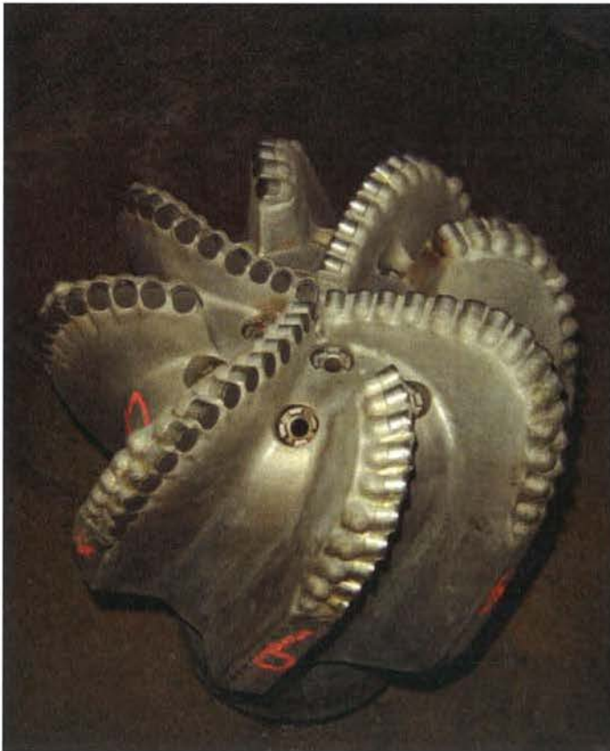
Figure 18: Dull Condition of PDC-A, after record setting run in Rawdhatain field. PDC-A, as shown above and developed with the new processes, achieved all the performance objectives set forth by the PTF.
