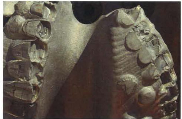
Figure 3: Impact damage to PDC cutters, as a result of severe bit vibrations.
