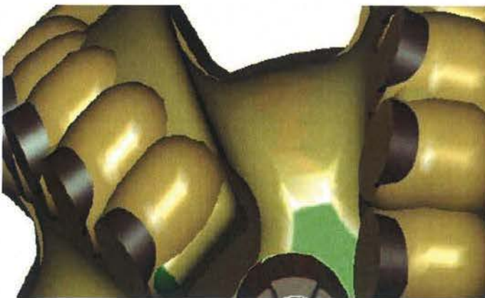
Figure 4: Section of PDC bit designed with low depth of cut (LDOC) feature.
