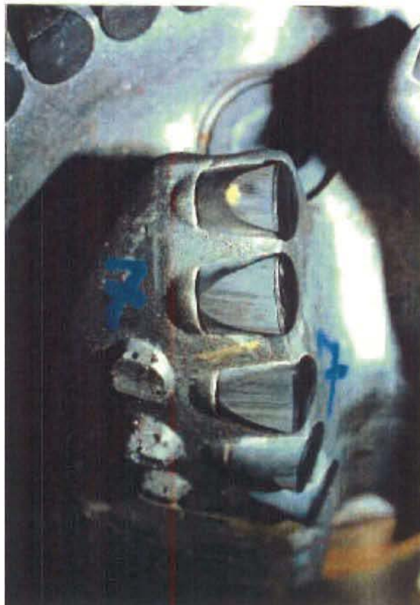
Figure 9 - Nose-to-shoulder dull of bit with standard PDC cutters – having drilled the same formations during 1993
