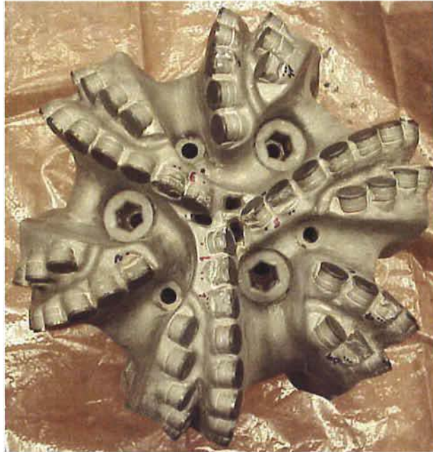
Figure 12 - Thermostable PDC bit dull condition after drilling the Mississippi Limestone
