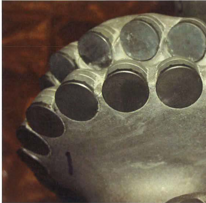
Figure 8 - Nose-to-shoulder dull of PDC bit with thermostable cutters
