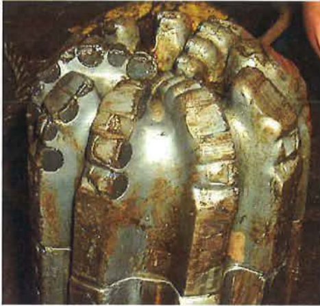
Figure 7 – Dull Picture of PDC-A after a successful run in the Rotliegendes formation on a turbo-drill.
