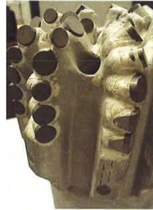
Figure 10 – Side view of NPDC bit, showing alternate orientation of different size cutters with different back rakes along a blade.
