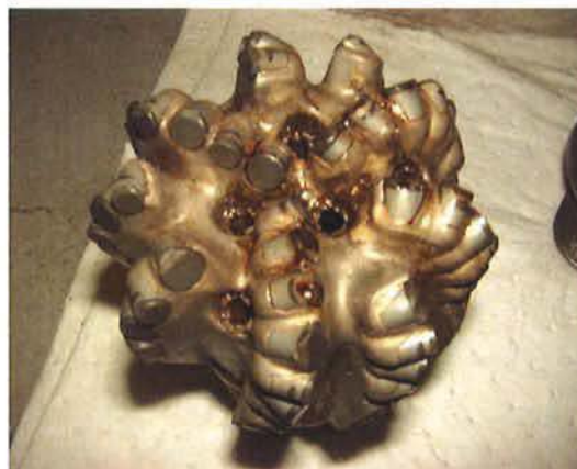
Figure 24 – Dull picture of 6" NPDC 1 , used in the hard, abrasive and conglomerate infested Hemlock formation in Alaska.
