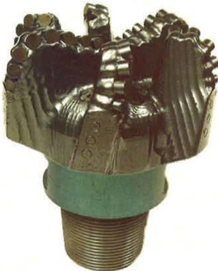
Figure 8 – PDC bit with maximized hydraulics performance parameter- open face volume, junk slot area and void volume ratio - for efficient cleaning and high penetration rates.
