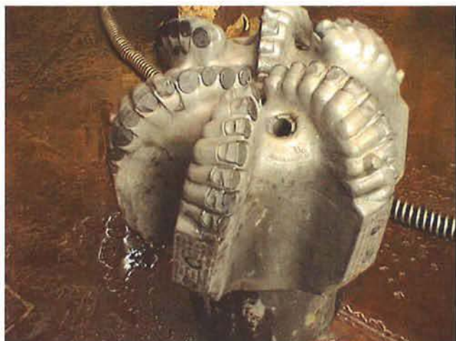
Figure 20 – PDC bit with relieved tungsten carbide substrate cutters after field run in abrasive formation. This specialized geometry reduces wear flat area, required WOB, and minimizes torque and heat checking.
