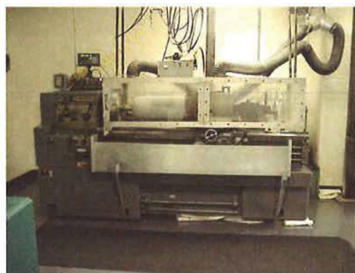
Figure 22 – Laboratory set-up used in testing specialized high abrasion cutters (PDC-A) and impregnated segments (IS). Samples were tested on Sierra white granite and Berrea Sandstone.
