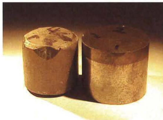
Figure 23 – Representative wear flat sizes generated on impregnated segments (IS) and specialized PDC cutters (PDC-A) during abrasion tests at identical conditions.
