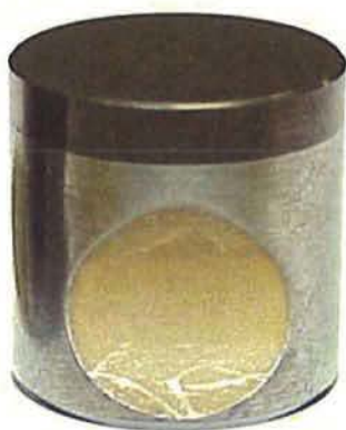
Figure 19 – PDC cutter with engineered relief in tungsten carbide substrate.
