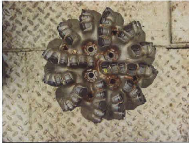
Figure 25 – Dull Picture 8-1/2" NPDC 2 , used in the Wyoming application to drill the Woodside, Dinwoody and Phosphoria formations.
