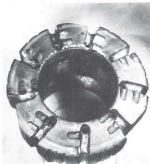
Fig. 16 – Style D core bit (no side rake).
