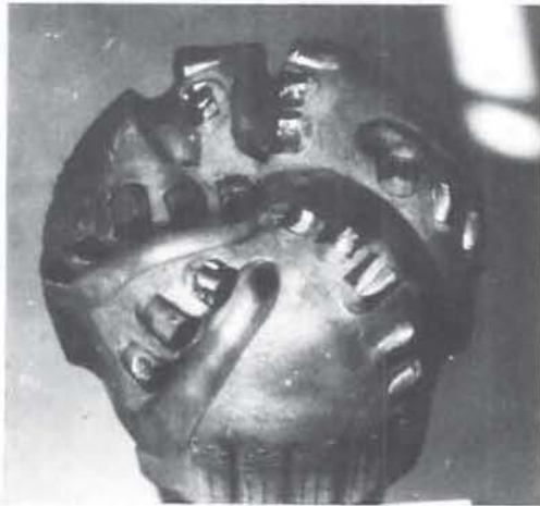
Fig. 14 – Style A drill bit (with side rake).
