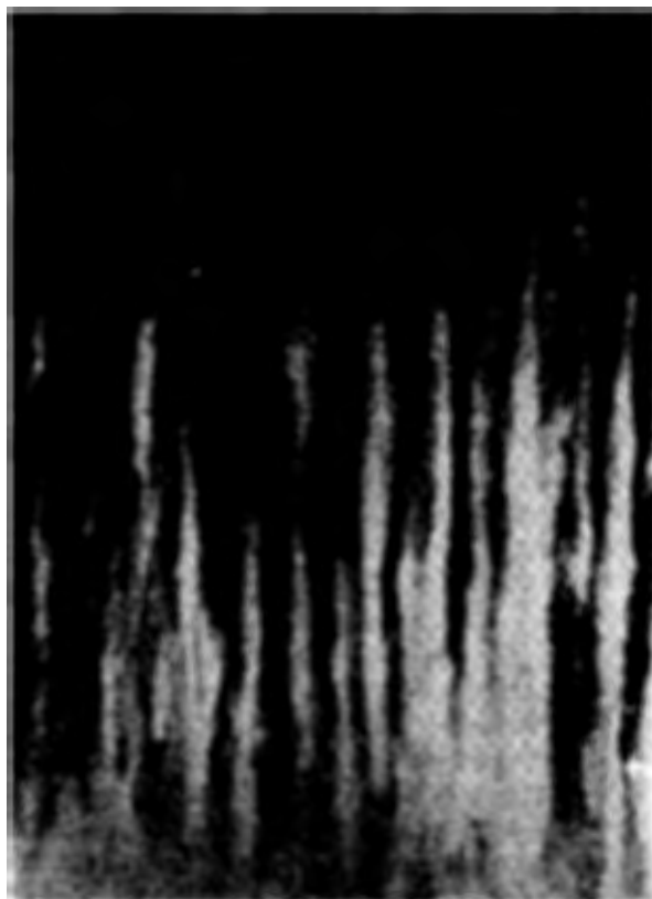
Figure 3 Vertical finger formation during sedimentation of a mixture of buoyant and heavy particles. The photograph was taken 60 seconds after mixing was completed, and the heavy particles are dyed. (From Weiland et al. 1984.)
