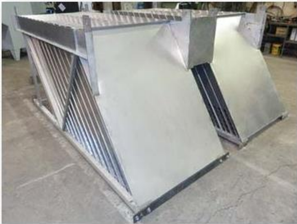
Example of parallel plates for sedimentation
