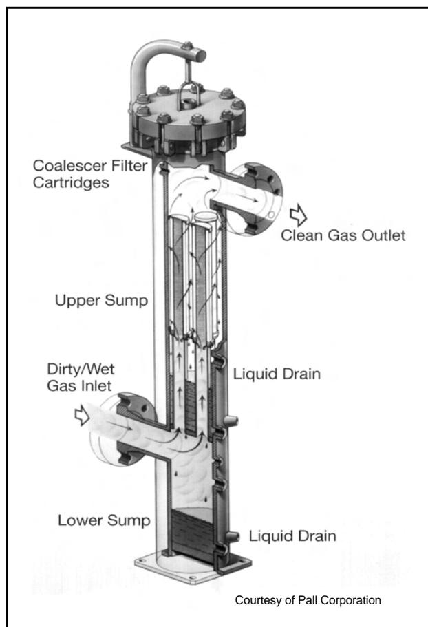
commonly refers to the removal of solids and liquids from a gas stream.
