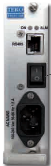
AC Power Supply Module
