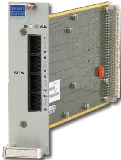
Alarm Board equipped with 16 input pins - TEA-I16
