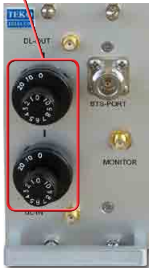
Passive POI with built-in duplexer
