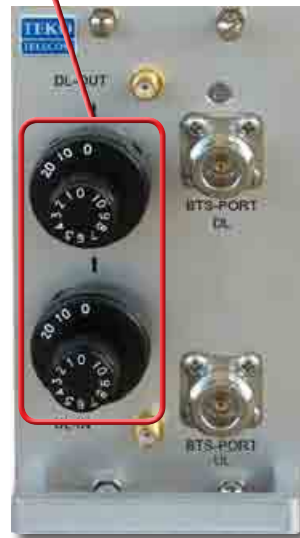
Passive POI without built-in duplexer
