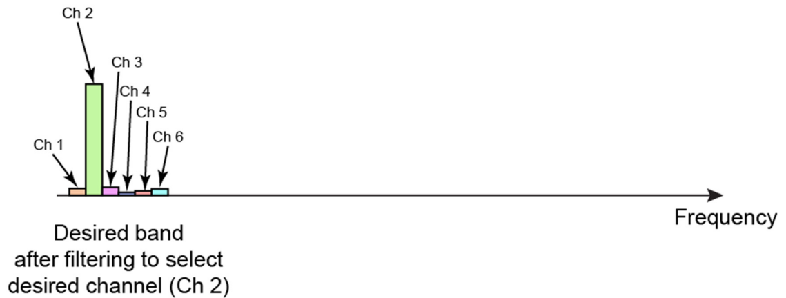
Figure 5. Frequencies in an input signal after the LPF attenuates all but one carrier.
