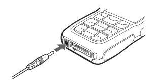
After a few seconds, the battery indicator in the display starts to scroll from bottom to top. If the battery is completely discharged, it may take a few minutes before the charging indicator appears on the display or any calls can be made.
