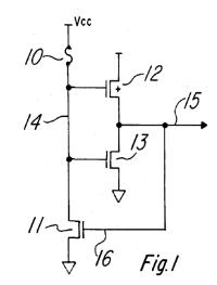
Figure 1 is an electrical circuit diagram of a CMOS fuse circuit according to one embodiment described in McAdams. *Id.* at 1:60–61. Fuse element 10 is
