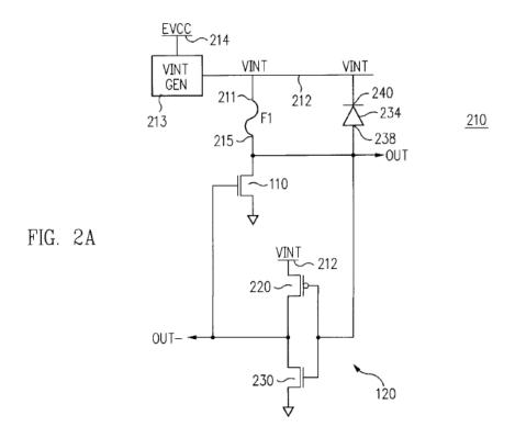
Figure 2A "is a circuit diagram of a programmable latch according to the present invention." Ex. 1001, 2:64–65. Figure 2A shows a programmable latch 210 including a fuse F1, NMOS transistor 110, CMOS inverter 120, VINT generator 213, and diode 234. As depicted in Figure 2A, CMOS inverter 120 is formed by PMOS pull-up transistor 220 and NMOS pull-down transistor 230. *Id.* at 3:24–26.
