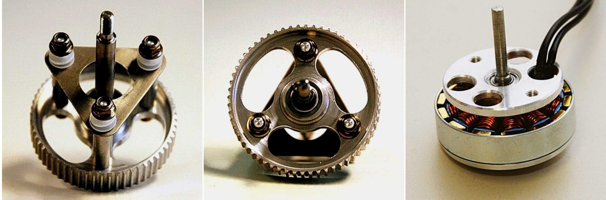
Figure 3.8: Top view (left) and bottom view (middle) of completely assembled rotor head and close-up view of 4-pole-pair 3-phase AC motor (right).
