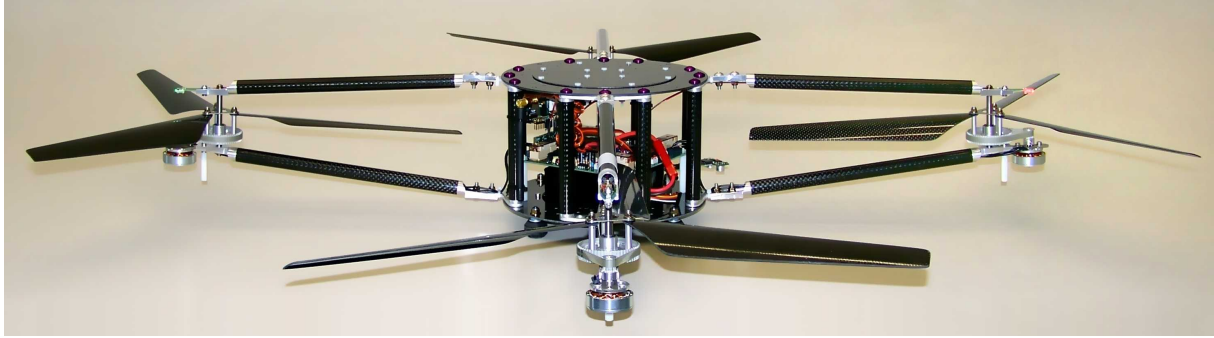
Figure 1.1: The JAviator quadrotor, a high-precision “aerial software testbed”.
